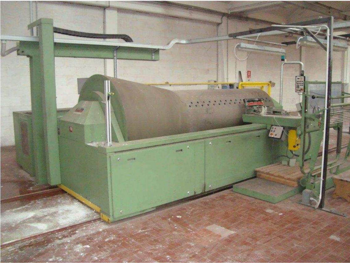
N°1 BENNINGER SECTIONAL WARPING MACHINE W:2200 YOC 1988 . WAXING DEVICE N°1 CREEL 320 BOBBINS GAUGE 27 MM
