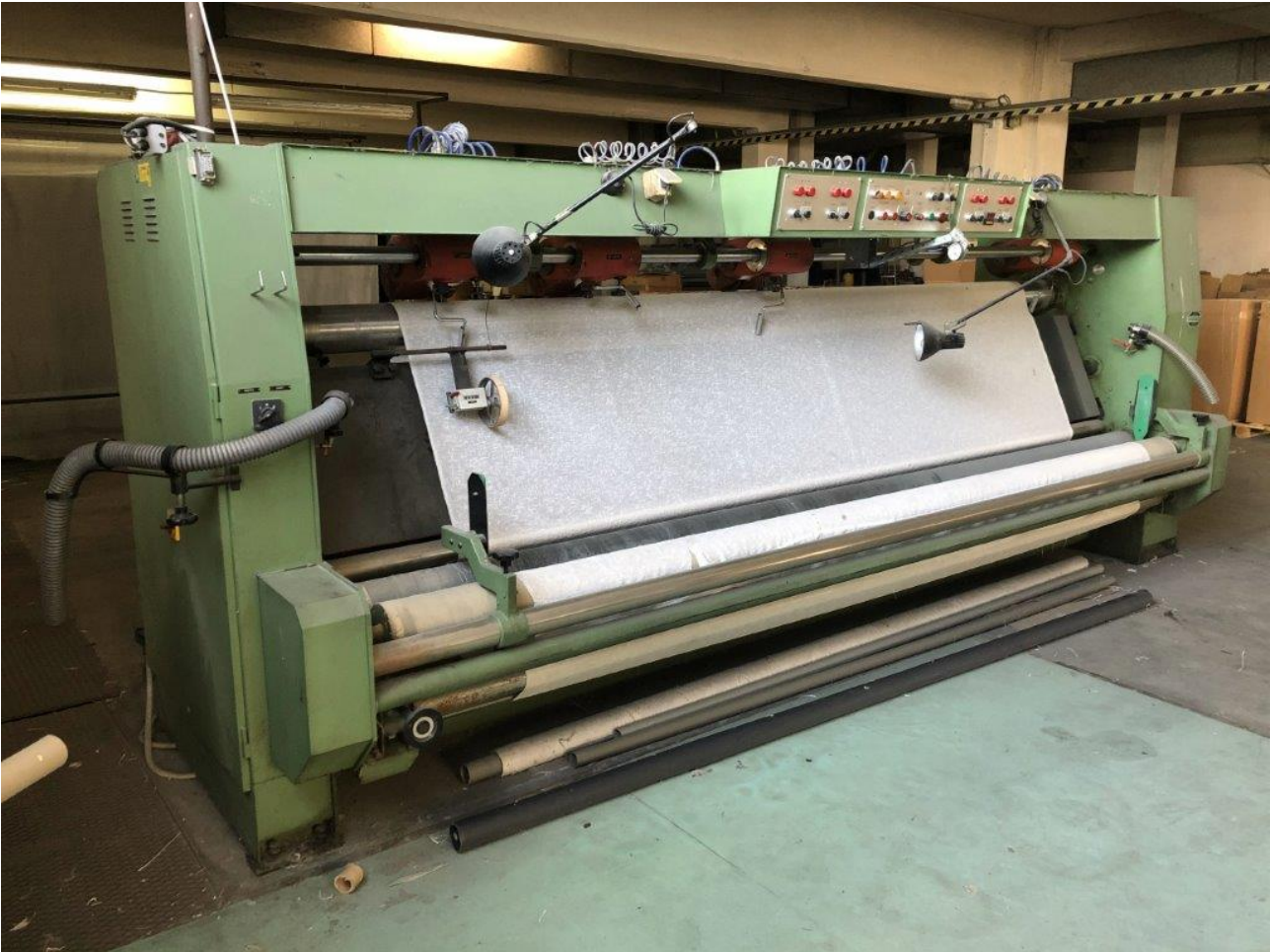
Nr.1 OFFRI THERMIC CUTTER MACHINE W:3800 YOC 1990 . 4 THERMIC CUTTERS
